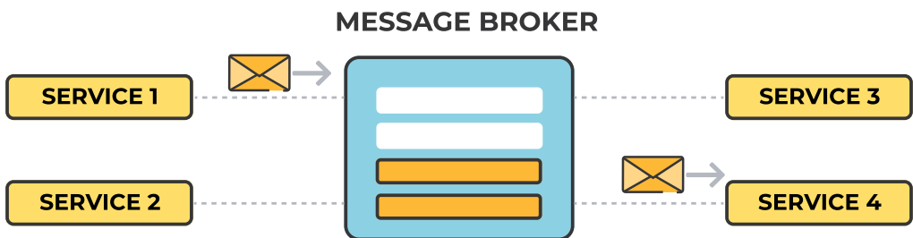
Figure 1 - Microservices exchanging messages via a message broker.
